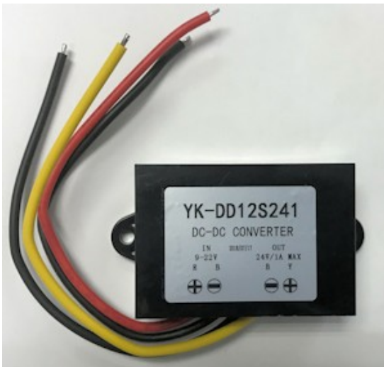
Photo 3: XA02-0046 DC to DC Converter
