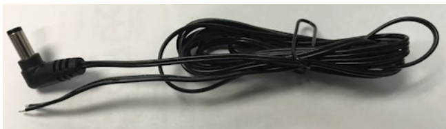
Photo 2A: Power Plug 5.5 mm diameter with 1 meter cable. The wire with Stripe is Negative,
