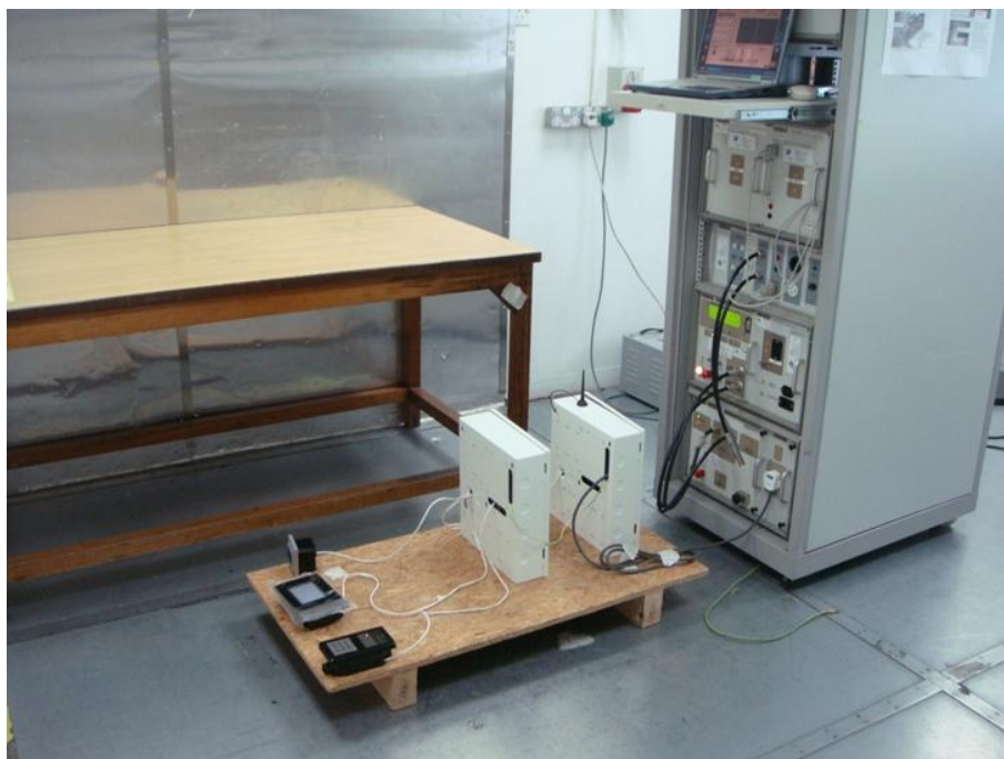
Voltage Surge Immunity Test Setup
