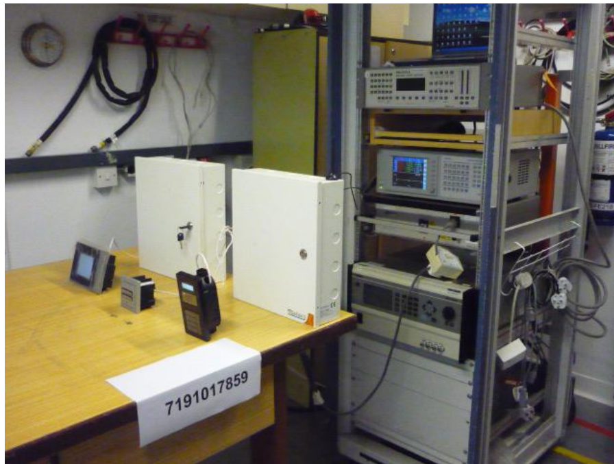
Voltage Dips and Interruptions Immunity Test Setup
