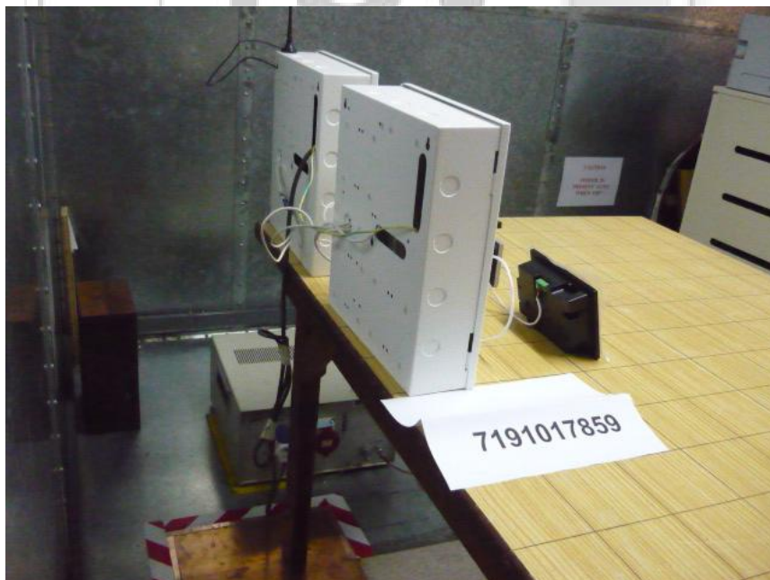
Conducted Emissions Test Setup (Rear View)
